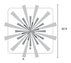
A: When walking across beam, detection will occur at approximately 22 feet. B: When walking into beam, detection will occur at approximately 12 feet.
